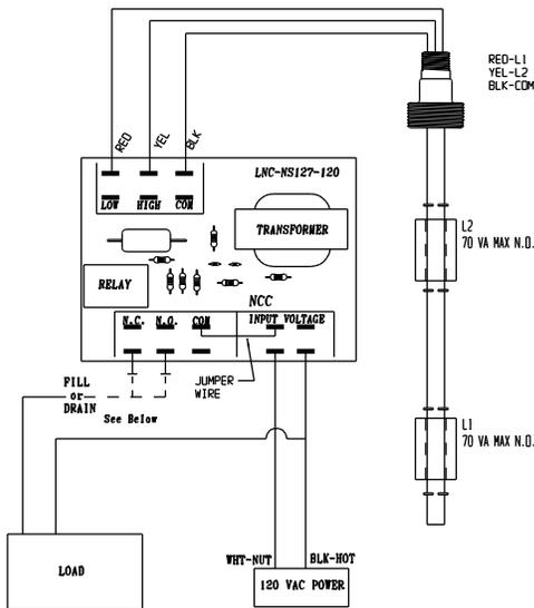
**DRAIN** WIRE TO N.O. CONTACT ON CIRCUIT BOARD:
