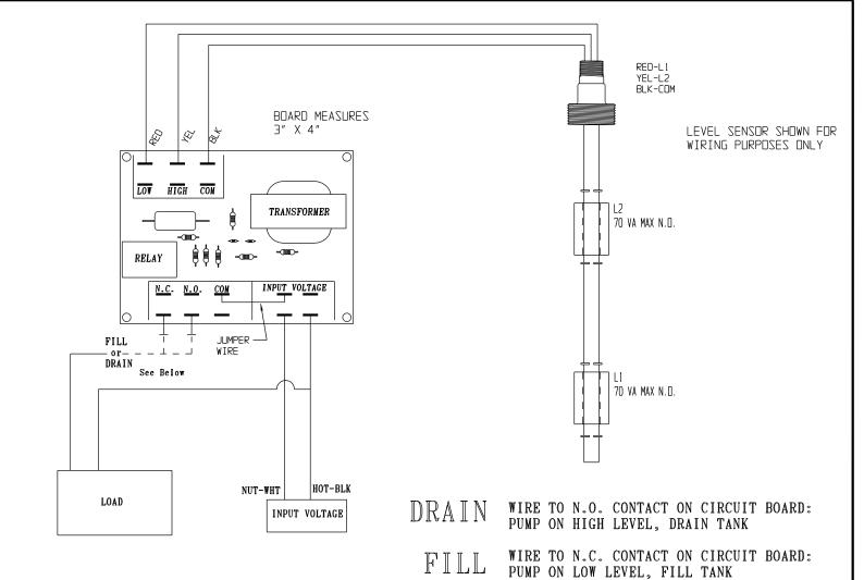
Liquid Level Control Relay for pump up or pump down applications
