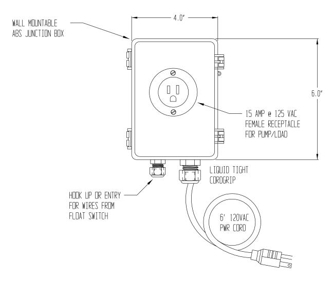
PUMP/LOAD ON WHEN FLOAT SWITCH CLOSES \*CONNECT LOAD TO PIN 3 OR 4
